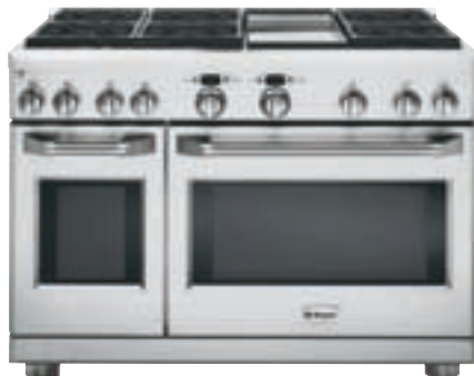
ZDP486NDPSS (natural gas) ZDP486LDPSS (liquid propane) 48" dual-fuel professional range with six gas burners and a griddle Dimensions: 47-7/8" W x 35-1/4"—36-3/4" H x 28-1/4" D
