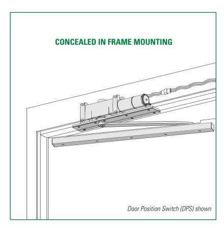
The concealed 2210 Series, heavy duty, high security track closer features complete concealment with special components to minimize tampering and vandalism. Forged steel, single lever arm and heavy steel mounting plate are designed for correctional, vandal prone, institutional, and other high traffic applications. A choice of finishes and cylinder functions meet correctional and vandal resistant requirements. **FEATURES**
