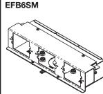
Module – Bank of three (3) compartments that accept power, communications and audio/video devices. Accepts standard size (2 3/4" x 4 1/2" [70mm x 114mm]) device plates. Includes device bracket, back plate, three (3) knockout plates (3/4"/1 1/4" concentric), two (2) end caps and one (1) divider.
