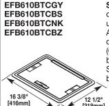
Surface Style Cover with Solid Lid - Die cast aluminum cover assembly designed to be used on top of floor covering. Available in the following powder coated finishes: black (BK), gray (GY), brass (BS), nickel (NK) and bronze (BZ). For use on Evolution Series 6-, 8- and 10-gang floor boxes (EFB6, EFB8 and EFB10).
