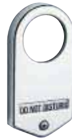
09-611 "Do Not Disturb" Indicator This unit is used with A or B design roses only. It requires a 1-3/8" (35mm) cylinder for 1-3/4" (44mm) doors. When ordering separately, specify finish. Specify L583-375 for "Occupied" indicator.
