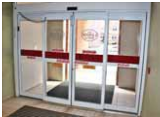
This GT 1175 bi-part automatic sliding entrance uses one-way activation and a magnetic lock for security. The automatic sliding door requires card access to enter. When employees and visitors leave the facility, they simply approach the interior sensor and the door opens automatically to allow egress.
