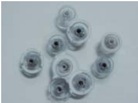
357 Magnum captured in Level 2 Polycarbonate
