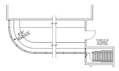
**San Diego Convention Center:** Manually operated panels create a security screen. Panels have perforated-steel, sound absorptive faces and paint finish.
