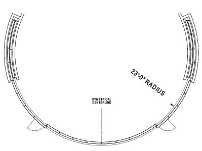
GE Capital: Bi-parting, electric operation, with four panel elements traveling on two parallel tracks. Welded steel panels with perforated, sound absorptive faces and paint finish.
