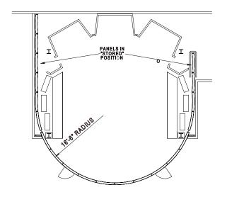
Osram/Sylvania Lighting Laboratory: Welded steel panels with fabric finish, powder coat trim, custom color seals and inset pass doors. Bi-parting wall is electrically operated with panels hinged in trains using "Soss" fully concealed hinges.
