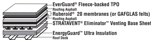
80 Mil Fleeceback Using EnergyGuard Ultra, With Your Choice Of Premium Ruberoid Or GAFGLAS Interplies
