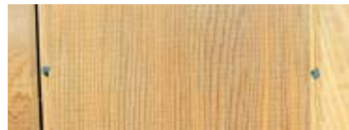
EXAMPLE OF SHRINKAGE IN A 1/2" THIN BOARD.
