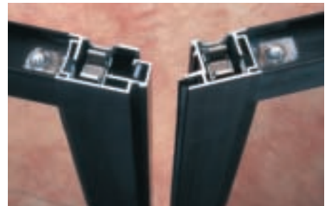
Panic Guard® Entrances Panic Guard® resists entry through the "security gap" between pairs of doors. When closed, a retracting aluminum astragal bar at the meeting stiles interlocks for the full door height. In addition, a continuous threshold stop and blade stops at jambs and head reduce the possibility of inserting hook wires under or around the doors. Guarded lock cylinders provide added security.
