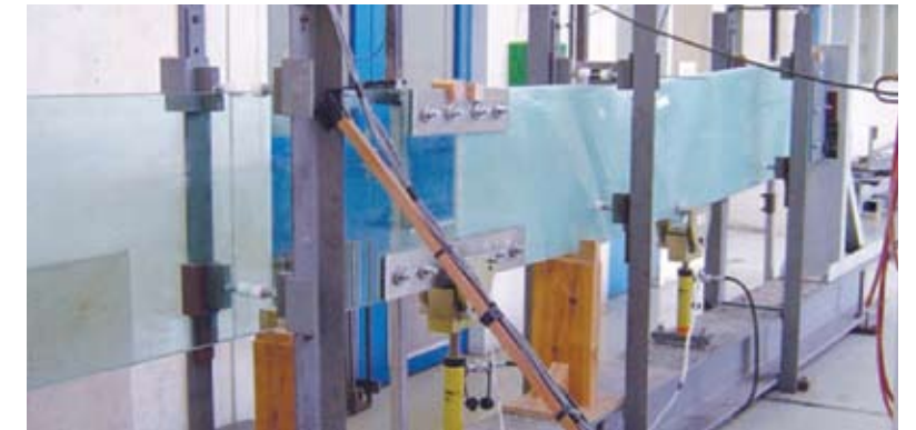
High Strength Laminated Fin Test
