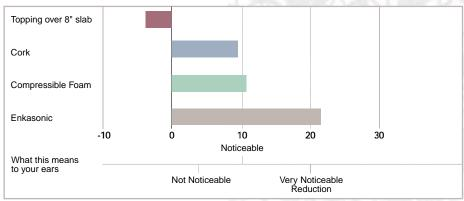
Note: Tests were performed with no ceiling assembly on 1'  $\times$  3' sample, marble thinset to a 4" slab.
